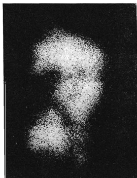
FIG. 7 Distribution of Vanadium in the Sample No. 15, Zdechovice (Magnif. 1500 \times )
