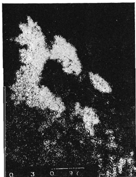
FIG. 10 Distribution of Sulfur in the Sample No. 2, Borovy (Magnif. 250 \times )
